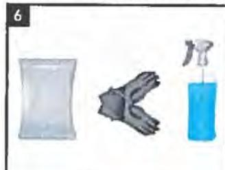
Water is needed to activate Wrapid Shield XL. Open the foil pouch, remove the roll. Once opened, the product cannot be repackaged. Wrapid Shield XL is activated using a water sprayer to mist and wet each layer as it is wrapped.
