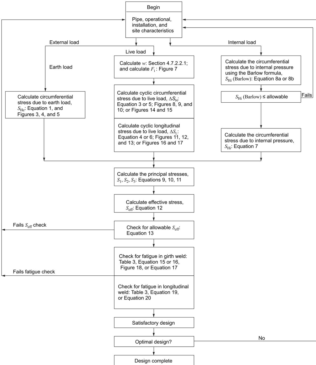
Figure 2—Flow Diagram of Design Procedure for Uncased Crossings of Railroads and Highways
