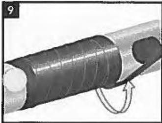
Apply compression film in the same direction as the previous layers with a 50% overlap. Start min. 50mm (2") beyond the outer edge of the Wrapid Shield XL, pulling firmly during application.
