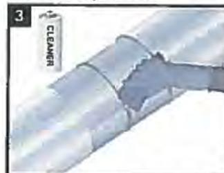
Clean exposed steel and adjacent pipe coating with an approved solvent (Acetone, MEK, Alcohol >96%) to remove the presence of oil, grease, and other contaminants if present. Ensure that the pipe is dry prior to mechanical cleaning.
