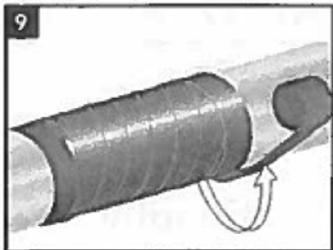
Apply compression film in the same direction as the previous layers with a 50% overlap. Start min. 50mm (2") beyond the outer edge of the Wrapid Shield XL, pulling firmly during application.
