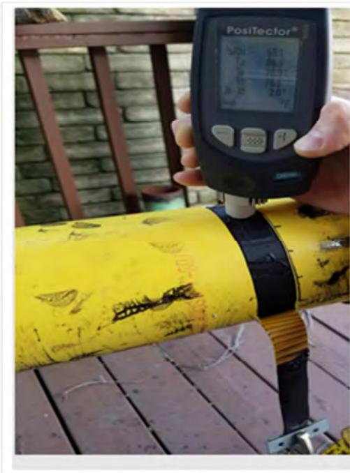
The testing and results obtained described above indicate that the Sleeve's performance was normal, acceptable and the peel testing in the field was conducted at a peel failure mode transition temperature (temperature differential). Both results would be considered a PASS.
