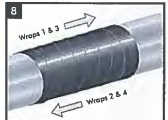
End with a circumferential wrap applied at 90° to the pipe. For high shear or impact requirements, additional layers may be required. To create thinned edges for directional drilling, reduce the overlap in the last 100mm - 150mm of the edges to 10-20% rather than 50%.
