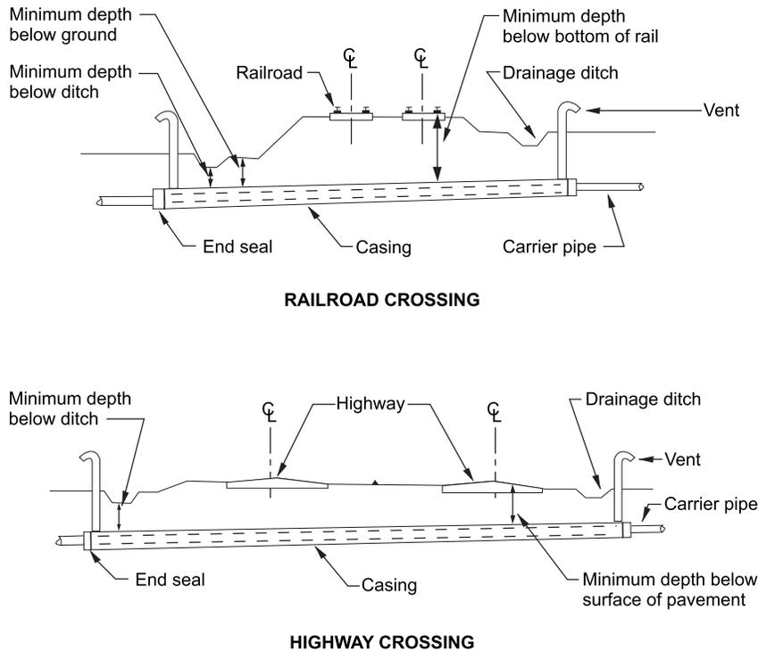
NOTE For simplicity, drawing does not include insulators/spacers (5.8 and 5.11) or test stations (6.3.6)
