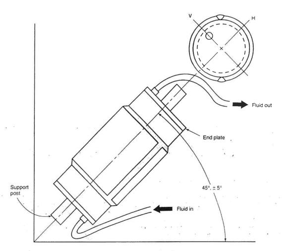
Note: This test position qualifies the procedure for all positions. Tests may be performed in other positions which will qualify the procedure for that position only.
