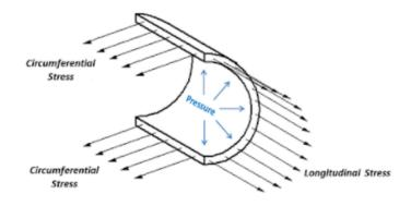
12 To calculate and evaluate the overall stresses acting on a pipeline, we account for the following
