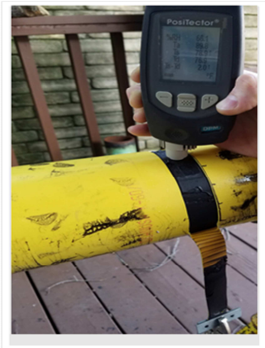
Figure 2: Follow Up Testing Canusa K-60/L, QA# 16-B-554.
