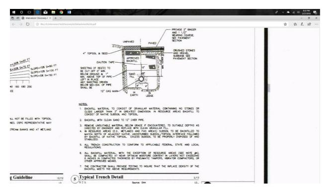
The diagram shows the pipe entirely surrounded by "SAND FILL." It shows a minimum depth of sand fill of 6" on earth trench bottom and 9" on ledge trench bottom. It shows 12" of SAND FILL above the pipe. Above the SAND FILL its shows "APPROVED BACKFILL."
