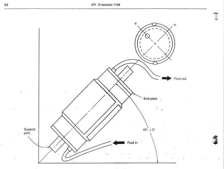
Note: This test position qualifies the procedure for all positions. Tests may be performed in other positions which will qualify the procedure for that position only.
