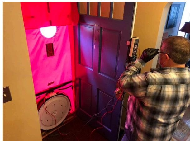
A VGS Residential Auditor preparing a blower door test on a home. The blower door test provides a baseline measurement for building heat loss. This test is conducted during the audit and after a project is completed.
