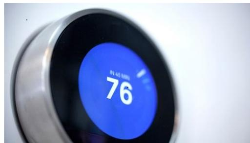
Smart thermostats provide customers with value on multiple fronts: easy time-of-day scheduling for desired temperatures and ensuring cost-savings during unoccupied periods.
